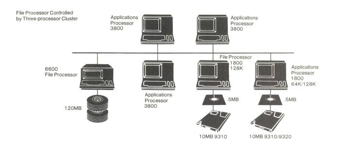
Figure C -- Using an 1800 as a Locally-Controlled Database
